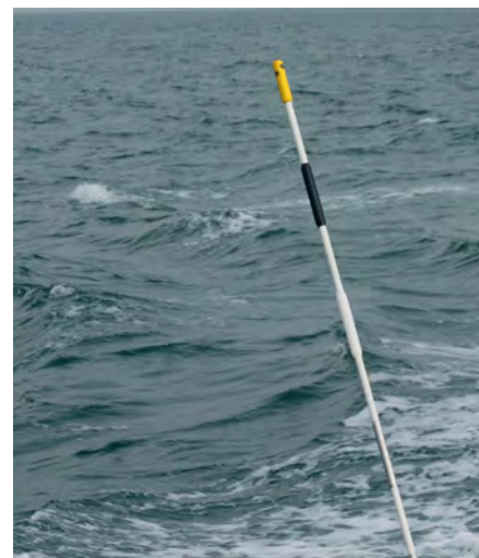
Figure 2. The Waverider buoy's HF antenna is an ideal location to integrate the air temperature sensor
