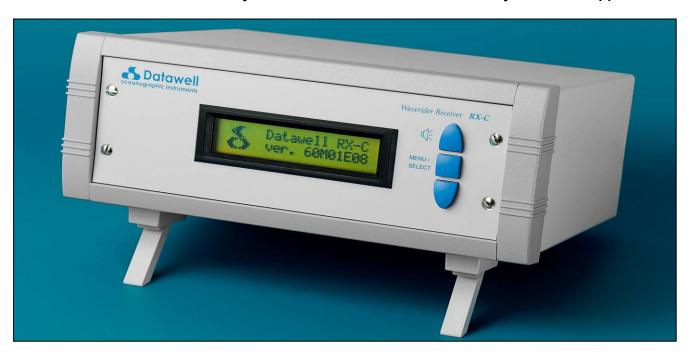
The RX-C is a dedicated HF link receiver that supports all Datawell Waverider buoys fitted with the standard HF transmitter. The RX-C supports both the "HXV" format and the "HVA" transmission formats. The HXV format is used by all buoys, except the DWR4(/ACM) buoy which uses the HVA format.
