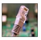
The Ethernet port makes the RX-C very flexible. The Ethernet port functions as four "virtual" serial ports. Once connected to a network or the internet, data can thus be
