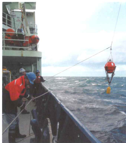
(Above) Fetch is packaged in a spherical pressure housing made from highly pressure tolerant and corrosion-proof glass. It has sufficient battery endurance for deployments of up to five years. (Below) Recent science cruises provided NOC scientists with their first opportunity to carry out tests on Fetch.
