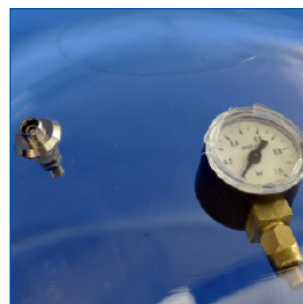
Vacuum port and manometer
